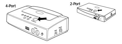
You can directly select a connected computer by pressing the Selector Button on the switch. The LED will be lit above the number to indicate which port is currently selected.
